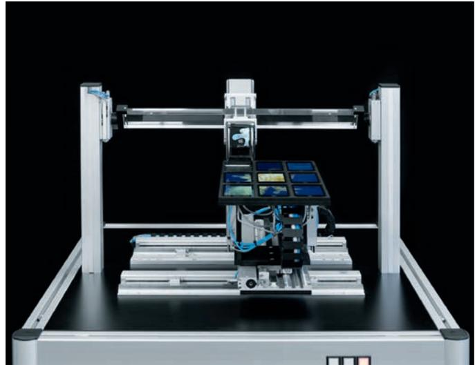
**Figure 2:** Energy-efficient grasping based on the model of the gecko foot setae: NanoForceGripper (Photo: Festo AG & Co. KG) [See more at: [https://www.festo.com/cms/en\\_corp/12756.htm](https://www.festo.com/cms/en_corp/12756.htm)]
